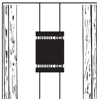
Slide flexible coupling over the pipe spigot ends of the two pipe.
