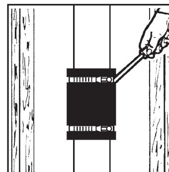
Tighten clamps to 60 inch-lbs. or torque.
